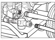
**Step 6** Disconnect the garden hose from the water inlet. Disconnect the high pressure hose from the high pressure outlet.
